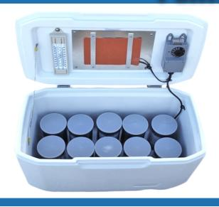
New economical way to protect concrete test specimens in the field. Thermostatically controlled to set it and forget it. Perfect for curing test specimens in all seasons.
