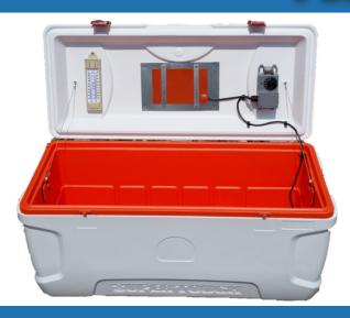
New economical way to protect concrete test specimens in the field. Thermostatically controlled to set it and forget it. Perfect for curing test specimens in all seasons.
